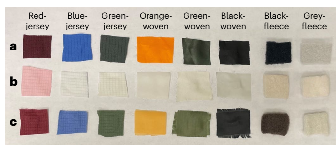
Fig. 5 | Overview of dye recycling. a–c , The PET fabrics in different stages: untreated ( a ), dye extracted ( b ), and redyed with the extracted dyes ( c ).
