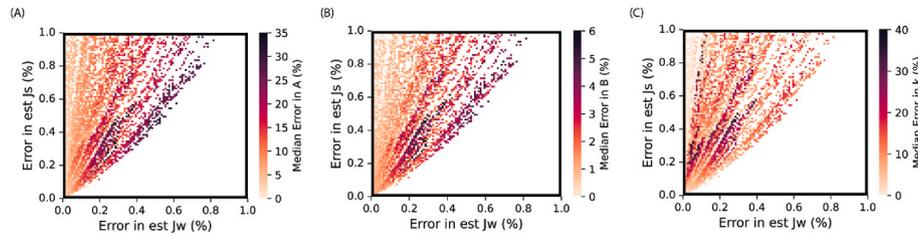
**Fig. 5.** Median error in the estimates of (A) water permeability, (B) salt permeability, and (C) mass transfer coefficient as a function of the absolute error in water flux and salt flux. The simulated result is generated using the pressure method in the pressure-sweep mode. The condition for the data simulation is outlined in Fig. 2.
